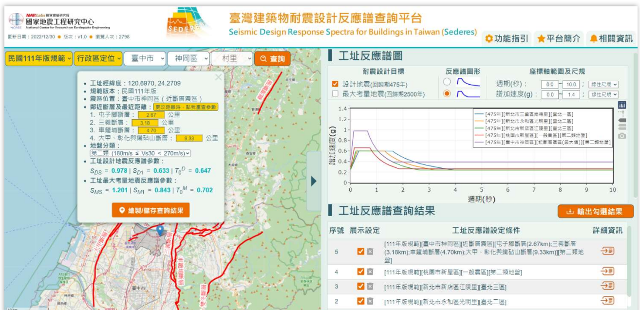
Fig. 1. The web service for seismic design response spectra for buildings in Taiwan (Sederes)
