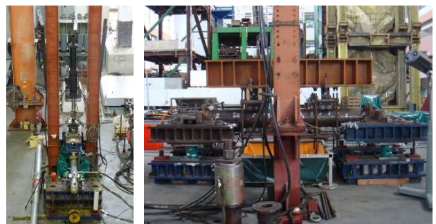
Fig. 2. Four-point bending tests of sprinkler piping joints (left) and NPP piping joints (right)
