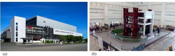
Fig.1. (a) NCREE Tainan laboratory. (b) The 8 m × 8 m shaking table and the three-story RC building (the white part).
