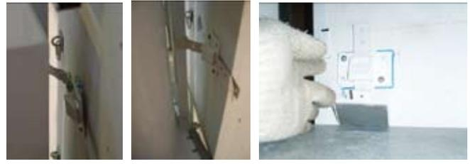
Fig.3 Failure of seismic restraint devices: pull out of expansion anchor (left), loosen belt (middle), and failure of adhesive layer attached on the table (right)
