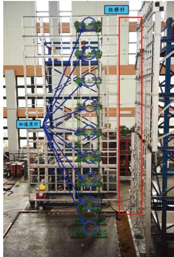
Fig. 1 LVDTs and accelerometers on the eight-story structure
