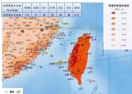
Fig.1 Seismic hazard map in China that has seven seismic design levels.
