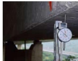
Figure 8: Micrometers to monitor girder displacement
