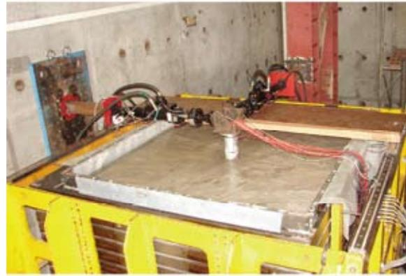
Fig. 1. Model pile pushover test
