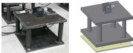
Fig. 1 Steel frame used in the shaking table tests.
