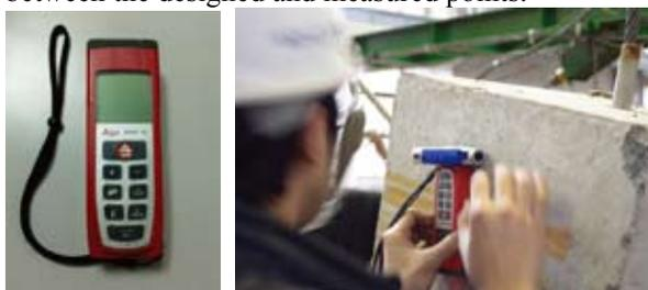
Fig. 8 Infrared gun used to measure distance
