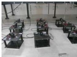
Fig. 2 For each contact surface condition, nine specimens were subjected to the input motions simultaneously.
