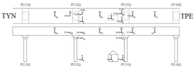
Fig. 9 Sensor configuration of the strong-motion monitoring station TAPBAA.
