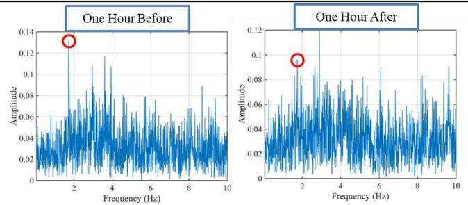
Fig. 11 Bridge frequencies before and after the 2022 01 03 earthquake.
