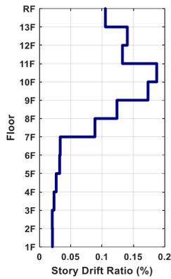
Fig. 8 Maximum interstory drift ratio of the NCREE office building in the X direction.
