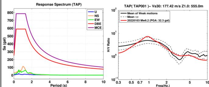
Fig. 5 Observed response spectrum and design spectrum (left) in three components from sample station TAP001, and its site transfer function H/V spectral ratio (HVSr) from shear wave windows (right). The black line indicates the average HVSr of historical weak motions, and could represent the linear site response; the red line represents this event.
