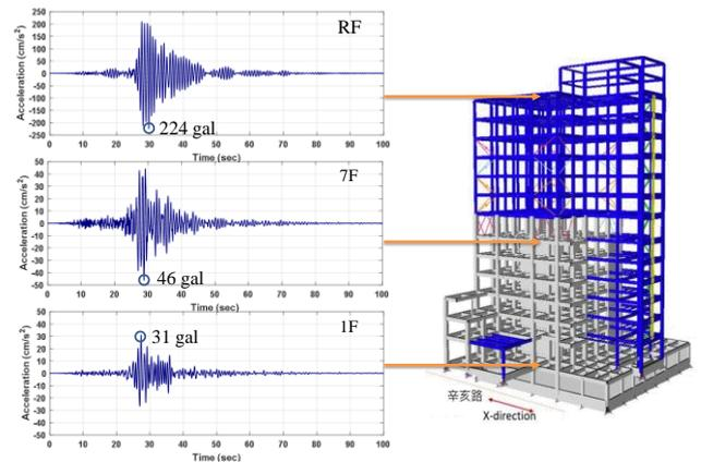
Fig. 7 Earthquake records of the NCREE office building. Grey: RC structure; blue: added steel structure.
