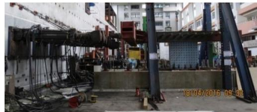
Figure 2. SC wall test setup.
