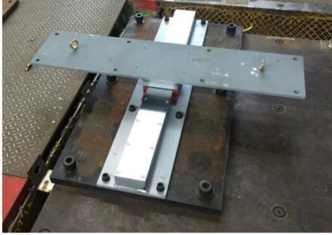
Fig. 1. The sloped sliding bearing model.
